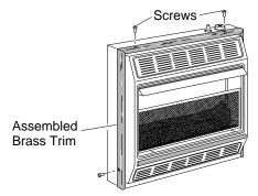
Figure 7 - Attaching Brass Trim to Heater
